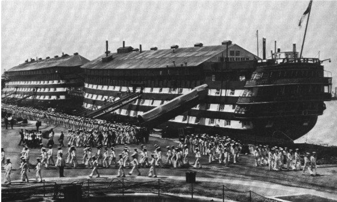
Two obsolete first-rates of the 1850s, Duke of Wellington (right) and Marlborough (left) spending their last years as depot ships at Portsmouth Dockyard. It is on record that to build HMS Duke of Wellington- 250 feet long with a 60-foot beam - an oak forest of 76 acres was cleared of trees. In this photograph, taken about 1898, a drum and fife band leads ratings ashore from the two hulks.
